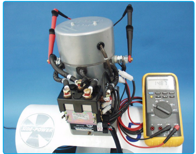
Checking voltage at thruster
