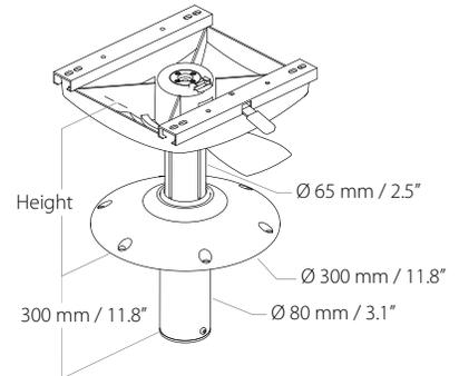
Fixed height seat pedestal with seat sliders and 360° swivel. The top can swivel freely and locks in the driving position.
