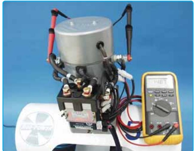
Checking voltage at thruster
