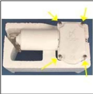
1. Begin by removing the 4 screws on the cover plate.
