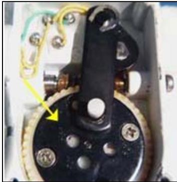
2. The sweep disc needs to be removed. This motor is pre-set in the 110° sweep angle.
