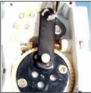
3. Begin by removing the circlip by using a screw driver or needle nose pliers.
