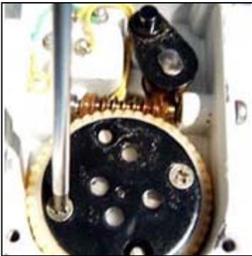
5. Unscrew the two screws fastening the transmission plate. (Be careful not to lose star washers.)
