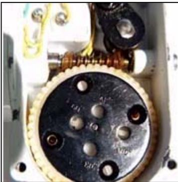
7. Place the transmission plate with the hole for the desired angle positioned directly over the groove for either L (Left Park) or R (Right Park).
