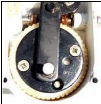
8. Replace transmission plate screws with star washers. Then reposition transmission arm and replace circlip back on to the transmission plate and refasten cover.
