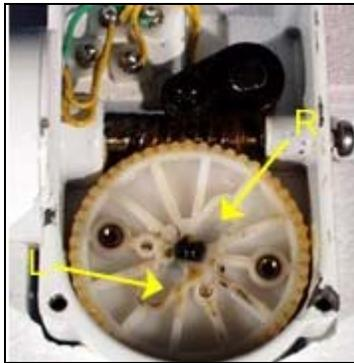
6. Remove the transmission plate from the white helical gear. Note the two grooves labeled L (Left Park) and R (Right Park).
