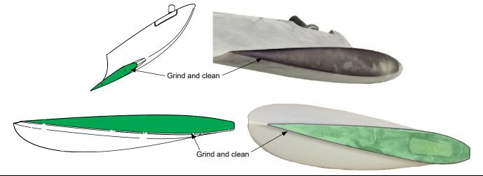
2. Proceed with a 'dry' installation of the winglet to the fin.
