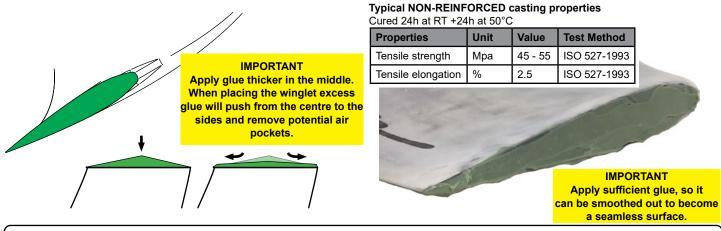
Place the winglet aligned with the fin surface. Lock and secure the winglet with previous screws to support the winglet and maintain pressure 4. during curing time. (NB: Especially if the fin is sitting on the boat.)
