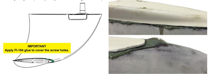
5. Smooth out the glue from the sides, holes and the front nose before its finished curing.
