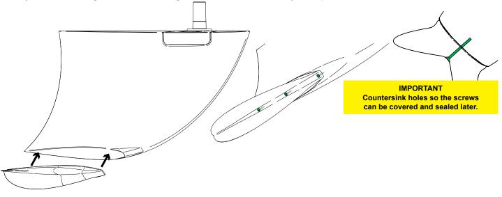
3. Remove the winglet. Apply a layer of the FI-184 glue to the correct surface of the fin. (See attached data sheet)
