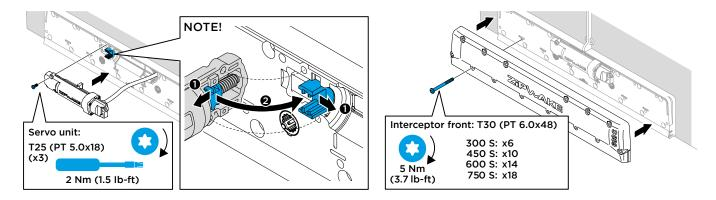
Instructions of mounting the SU-S and the front to the backplate. Ensure screw shaft nut is fitted correctly to the backplate's connecting rod. Tighten the screws with designated torque (2 Nm and 5 Nm, respectively).
