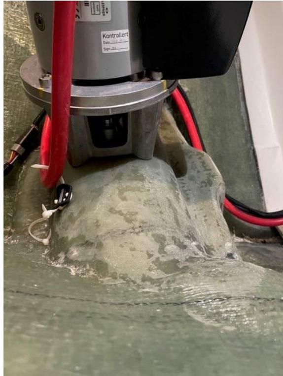
*The result of misalignment is premature wear of the drive coupler, and it will break depending on use and not as the product was intended. Damage to a coupler or any resulting damage to any other components or equipment, is not covered under the product warranty*
