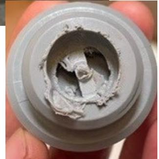
The result of misalignment is premature wear of the drive coupler, and it will break depending on use and not as the product was intended. Damage to a coupler or any resulting damage to any other components or equipment, is not covered under the product warranty.
