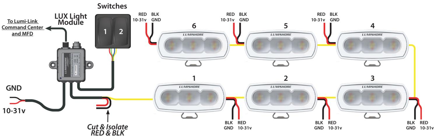
**Note : Black wire from each light and LUX Module should connect to common ground**
