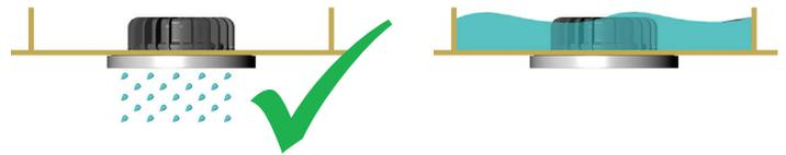
Also, it is important that the lights are mounted with airspace around the heat sink housing to allow for convective cooling of the lights. We recommend a distance of 1/2" (13mm) of free space above the housing.
