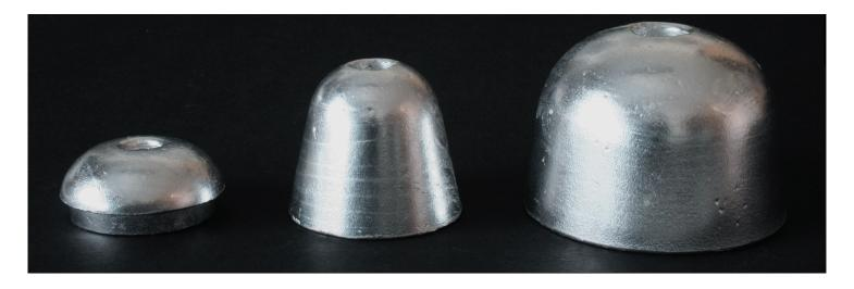
The alloy used in our Al-Zn-In anodes is quite different to normal aluminum. The mil-spec alloy includes about 5% Zinc and a trace of Indium to prevent oxidation resulting in a layer reducing the sacrificial properties of the anode.
