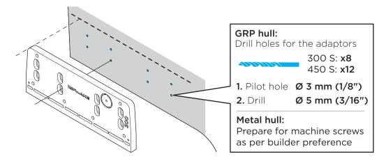
**3. Prepare the transom for optional concealed thru-hull fitting NOTE!** For thru-hull fittings above the waterline go straight to step 4!
