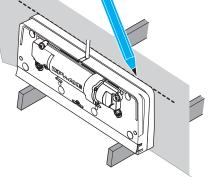
**NOTE!** Protruding hull: Cut off the lower edge of the adaptor with a right-angle grinder if necessary!
