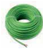
732I/100 Due Fili Plus cable for internal/external laying, 2x1 mm 2 twisted conductors, LSZH sheath and insulation, operating temperature -25/+70°C, insulation degree 600/1000 V, suitable for laying underground in dry ducting or channels with efficient drainage (max. 24 hrs wet), not suitable for laying directly underground - 100 m bundle
