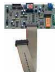
01708 PSTN communicator for control panel
