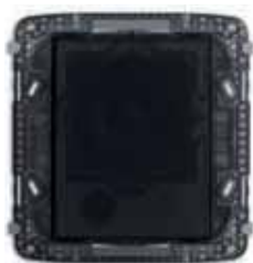
21588 Passive speaker, 8 Ω 10 W, with built-in 8-module mounting frame. Depth: 48 mm
