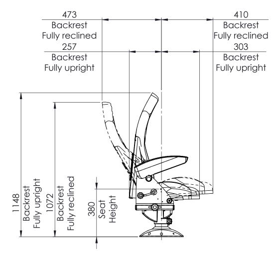
All sitting heights measured without load a variation may occur depending on the load due to contraction of gas-struts, springs, upholstery and third part equipment. All information herein contained is subject to change without notice unless under contractual configuration control.
