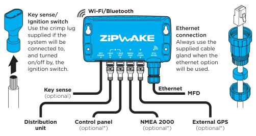
\* IMPORTANT The integrator module requires at least one external GPS signal via MFD, NMEA 2000, Zipwake control panel or Zipwake external GPS.
