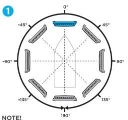
Make sure the integrator module orientation angle (mounting angle relative the boat's forward direction) is set as accurately as possible (±5°) during initial start-up.
