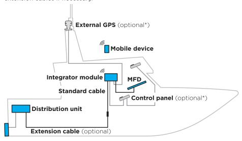
With the integrator module connected, the system can be controlled from one or several sources e.g. an MFD, a mobile device or a Zipwake control panel.
