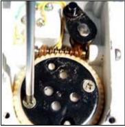
Unscrew the two screws fastening the transmission plate. (Be careful not to lose star washers.)
