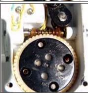
Place the transmission plate with the hole for the desired angle positioned directly over the groove for either L (Left Park) or R (Right Park).
