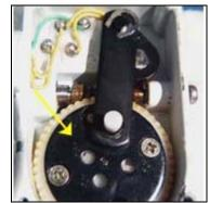
The sweep disc needs to be removed. This motor is preset in the 110° sweep angle.
