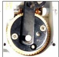
Replace transmission plate screws with star washers. Then reposition transmission arm and replace circlip back on to the transmission plate and refasten cover.
