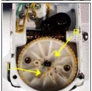
Remove the transmission plate from the white helical gear. Note the two grooves labeled L (Left Park) and R (Right Park).
