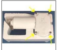
1. Begin by removing the 4 screws on the cover plate.
