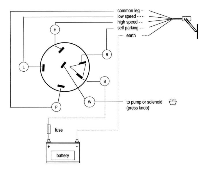
Please refer to the instruction manual as supplied with the wiper motor for appropriate motor wiring.
