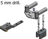
Re-assemble the blade clip in-between washing jet and T-piece, with supplied fasteners.
