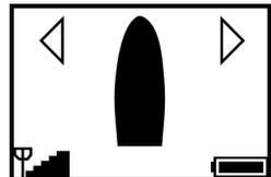
▽ Press the down button to return to stern thruster operation.
