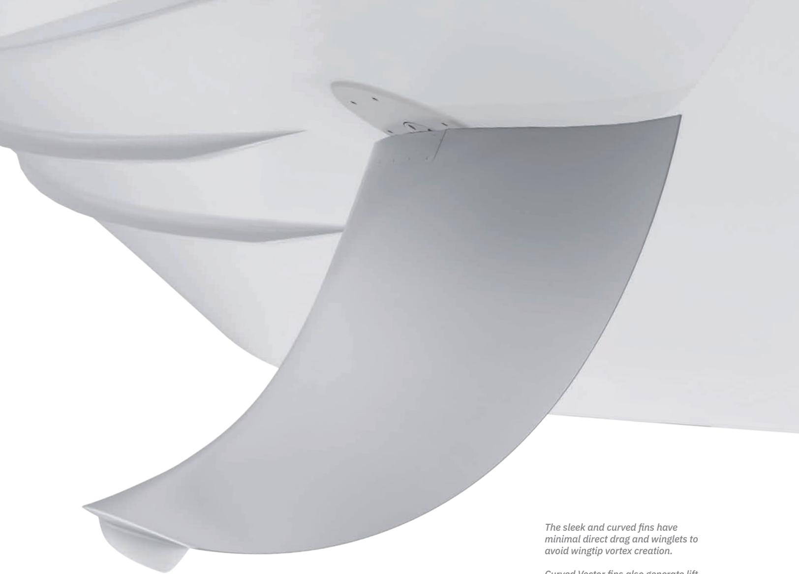
*The sleek and curved fins have minimal direct drag and winglets to avoid wingtip vortex creation.*
