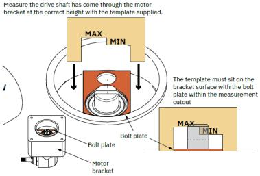
See pictures on page two on Visually checking driveshaft/leg in motor mount.
