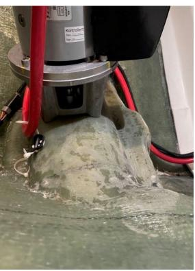
The result of misalignment is premature wear of the drive coupler, and it will break depending on use and not as the product was intended. Damage
