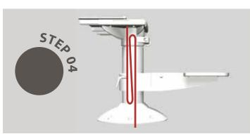
For NorSap 800 chairs, the wire will not fit inside the column and needs to be placed on the outside. The wire should go thru the plastic ring on the side of the footrest. See last page for flange modifications regarding the 800 series of NorSap chairs.
