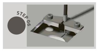
Place the chair on the wagon of the basic deck rail - use a piece of cardboard for protective measures when tilting the chair to gain access to the wire.
