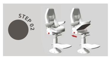
Remove the hand wheels on the side completely and push the seat frame backwards until you gain access to the center of the column.
