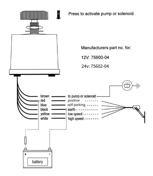
Please refer to the instruction manual as supplied with the wiper motor for appropriate motor wiring.
